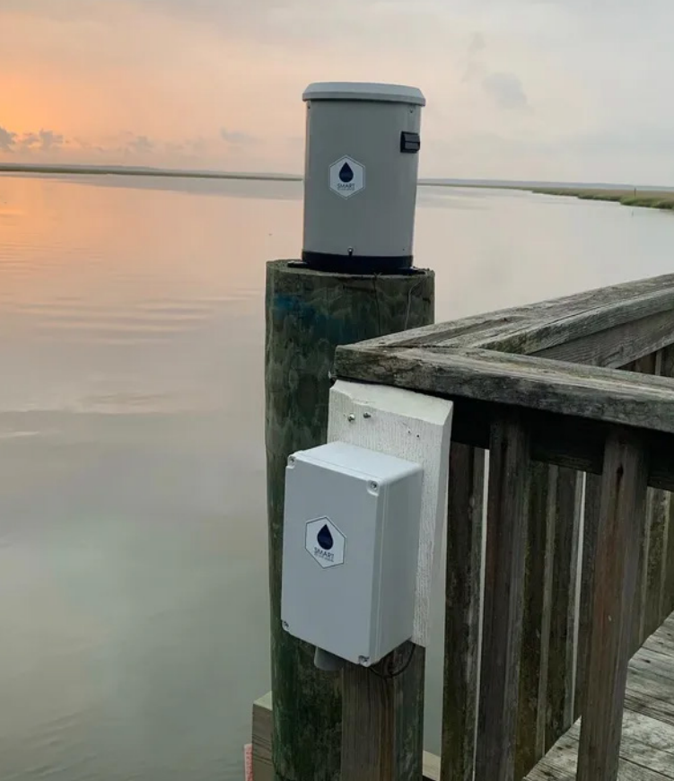
A "tipping bucket" rain gauge (background) is wired to a sea level sensor (foreground). RUSS CLARK
