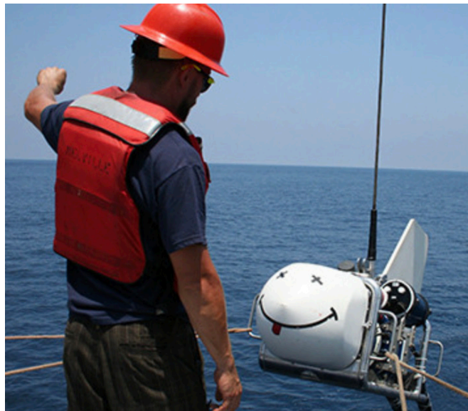
Researchers deploy an electromagnetic transmitter to study plate tectonics during a 2010 research expedition off the coast of Nicaragua. STEVEN CONSTABLE, SCRIPPS INSTITUTION OF OCEANOGRAPHY
